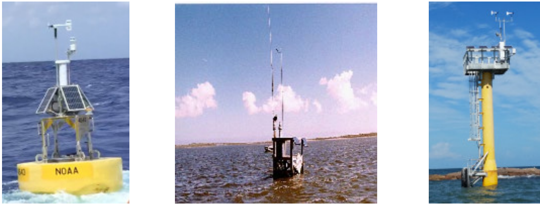
Figure 3-2. (left to right) NDBC Stations 42020, RSJT2, and ANPT2 with anemometers located at heights of 4, 10, and 14.22 m above sea level.
