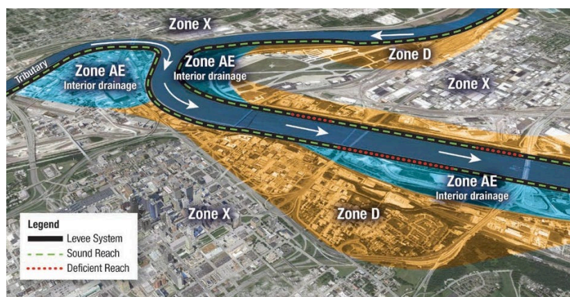
Figure 1. Example of new Zone D flood hazard areas behind a freeboard deficient reach
