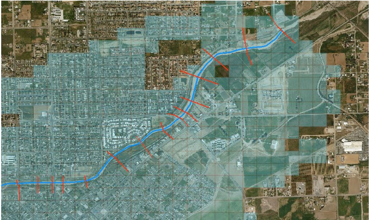
Figure 11-1: Example of an inundation delineation directly from a two-dimensional model (red lines on the graphic represent cross-section locations)
